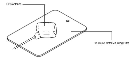
Position the GPS antenna in the center of the vehicle at the highest point with a clear view of the sky.
