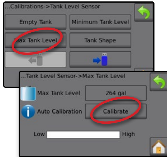
Figure 37: Tank Level Sensor – Maximum Tank Level
