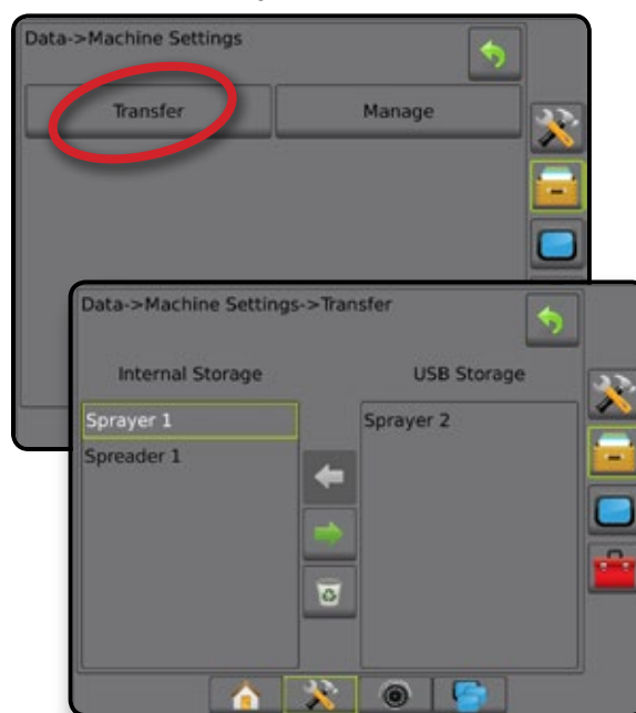
Figure 4-38: Machine Settings – Transfer
