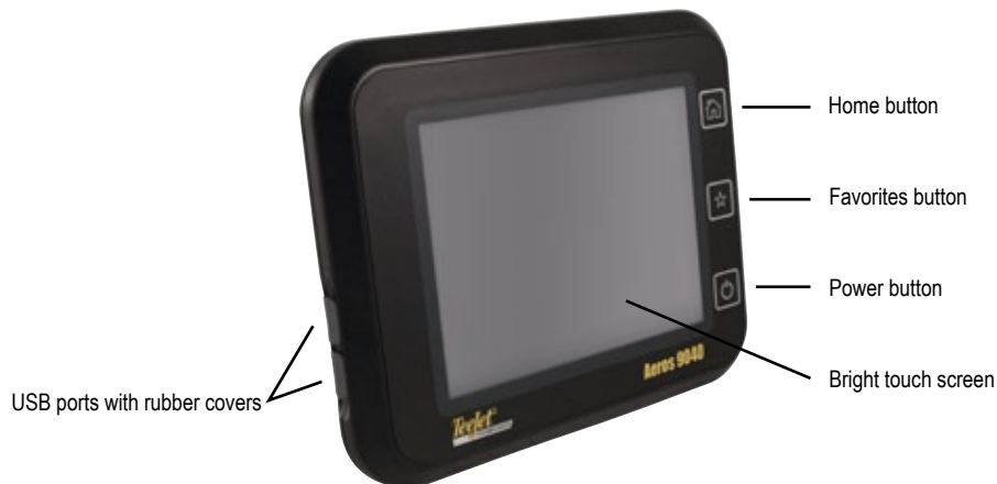
Figure 1-1: Aeros 9040 console front
