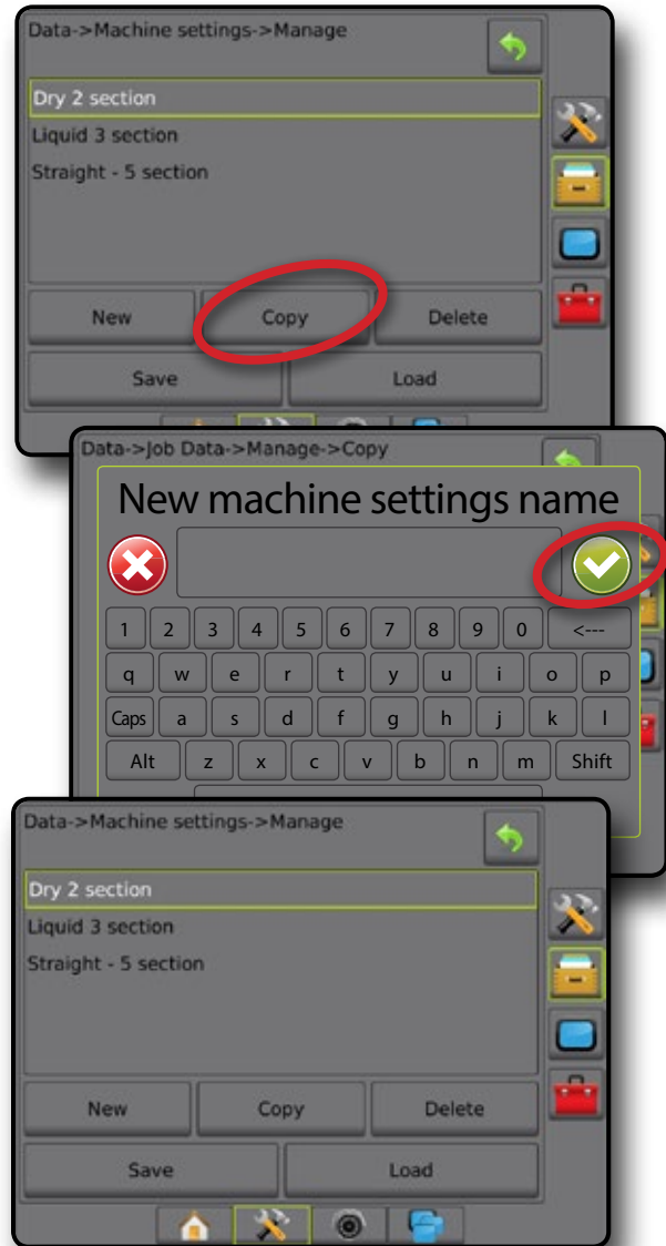
Figure 4-40: Machine settings – copy profile
