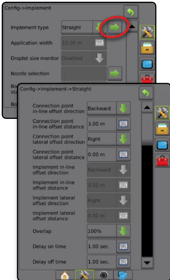
Figure 6-29: Straight implement type with ISOBUS Sprayer
