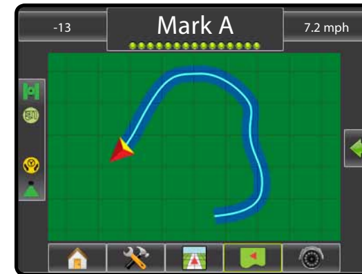
Figure 1-9: Boundary in Progress
