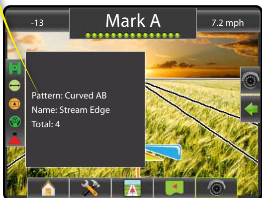
Figure 1-14: View Which Guideline is Active
