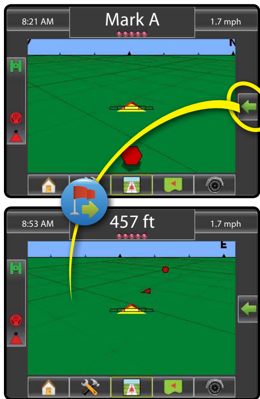
Figure 1-12: Return Point Established - Vehicle View
