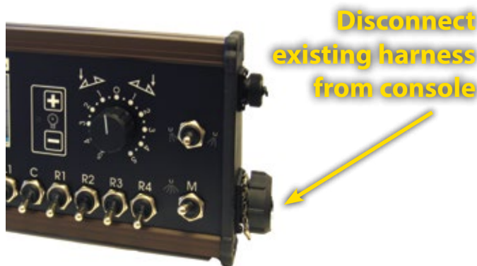
Figure 6: BoomPilot harness to flow control harness
