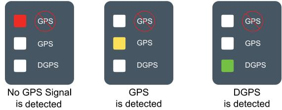
If the DGPS light is flashing, communication has been established with the GPS source; however, NMEA output rate is too slow. Ensure proper NMEA message settings of 5 GGA in the GPS device. Application cannot occur until proper communication is established.
