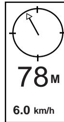
Press the Return to Point key to establish a point in memory. Normal guidance will continue uninterrupted during this process.
