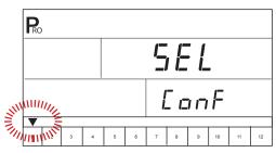
Press the Auto/man 😁 key to setup the reference pressure and reference flow of the selected preset.
