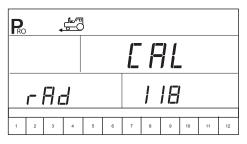
Drive toward the initial point of the designated 100 metres. At the starting location, press the Plus 🛨 key once to begin the calibration process. Continue driving the course. The 844-AB will count the impulses as the sprayer moves. The speed at which the vehicle travels is not important. As the ending point is reached, press the Plus 🛨 key again. The console will display the radar speed calibration number.
