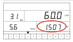
NOTES: The area counter/volume measure works only when the Master boom switch is in the "On" position.
