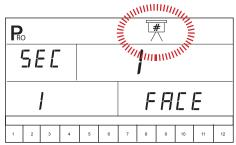
Use the Plus 🕀 or Minus 🗁 keys to adjust the value. This step will repeat for each section. Press the Programme 🗷 key to advance to the next section. The number of sections available is determined within the OEM setup options.
