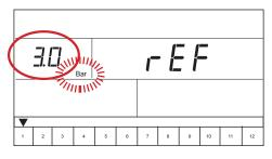
Press the Auto/man ↔ key to advance to the reference flow for current preset section.
