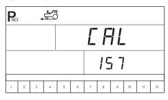
NOTE: Once the automatic speed calibration process has been activated, no other functions will operate until the console receives speed impulses for calibration. To deactivate automatic calibration mode, press the Plus 🗈 key twice.
