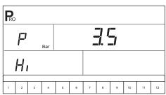
NOTE: If a pressure transducer is not installed on the system, skip this step by pressing the Programme R key. Leave the default value at "10 Bar".
