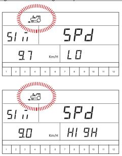
To enter simulated speeds, determine whether the low or high simulated speed is displayed on the console. Change from low to high by pressing the Auto/man 🕶 key.
