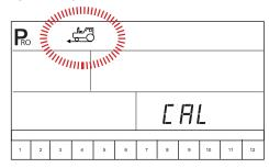
Drive toward the initial point of the of designated 100 metres. At the starting location, press the Plus key once to begin the calibration process. Continue driving the course. The 844-AB will count the impulses as the sprayer moves. The speed at which the vehicle travels is not important. As the ending point is reached, press the Plus key again. The console will display the speed calibration number.
