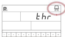
NOTE: Once the throttling mode is selected and the console is set to "manual" mode, the pressure regulating valve should open when the Plus ⊕ key is pressed and close when the Minus ⊖ key is pressed.
