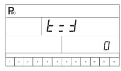
Press and hold the Programme R key for three seconds to exit System setup mode. Changes will be saved to the console's memory.
