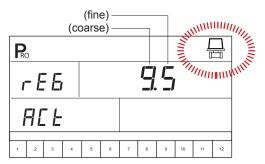
If the regulating valve is plumbed in the throttling position (supply line), start with a valve speed of 3.0 and adjust the number according to application requirements. Adjusting agitation volumes can often assist the regulating valve operation. Press the Programme Reverse to accept the entry and advance to the next step.
