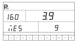
Once the display finishes counting, a number close to 4.0 (+/- 0.2) should be displayed. The low pressure value of the transducer is calibrated. Press the Programme R key to advance to the next step.
