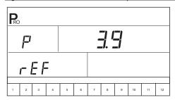
NOTE: If a pressure transducer is not installed on the system, skip this step by pressing the Programme R key. Leave the default value at "4.0".
