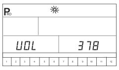
Press the Programme R key to return to the Setup mode. The new flow meter calibration number will be displayed. To accept the value displayed, press the Programme R key again. To repeat the calibration procedure, repeat the previous steps.
