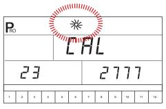
Press the Programme B key. The console will ask for the volume that was sprayed. Use the Plus H or Minus  $\boxdot$  keys to adjust the value to match the volume sprayed in litres.
