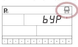
NOTE: Once the bypass mode is selected and the console is set to "manual" mode, the pressure regulating valve should close when the Plus key is pressed and open when the Minus key is pressed.
