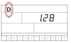
NOTE: If a liquid with a density other than water will be sprayed, and that density was programmed into the Specific gravity (Density) step during System setup mode, the "D" symbol must be selected during Application setup mode to activate the alternate density.
