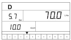
After performing the calculations, advance to the beginning of Application Setup mode to make changes by pressing the Programme key. If no changes are necessary then Application setup mode is complete. Press and hold the Programme key for three seconds. Changes to Application setup mode will be stored in the console's memory.
