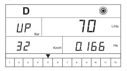
To return the application rate to the original target rate, use the Plus ⊕ or Minus ⊖ keys individually to increase/decrease the rate in 10% increments, or press the Plus ⊕ and Minus ⊖ keys simultaneously to return to the programmed target application rate.
