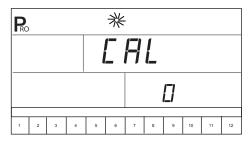
Engage the sprayer pump. Turn the boom sections "On" and begin spraying a known volume of fluid (e.g. 400 litres). As the known amount is sprayed, the console will count the impulses. After the known volume has been sprayed, turn the Master switch "Off" to stop counting impulses.
