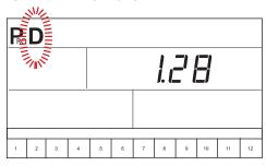
Use the Plus 🛨 or Minus 🗆 keys to change the value. Press the Plus 🛨 and Minus 🗆 keys simultaneously to clear the value to "0". Press the Programme 🖻 key to accept the value and advance to the next step.
