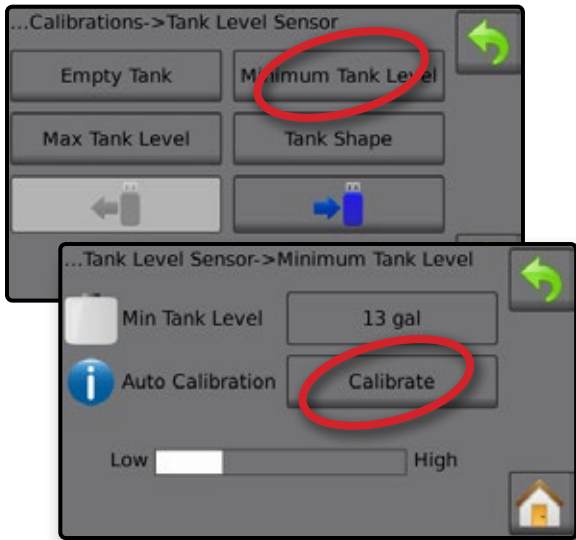
Figure 3-28: Tank Level Sensor – Minimum Tank Level
