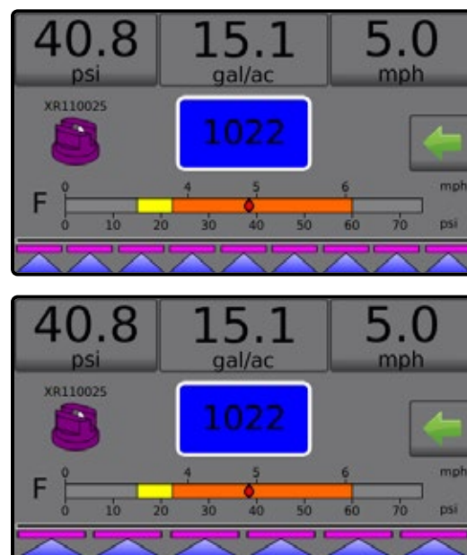
Figure 3-37: Operation Screen with 9 or 6 Sections
