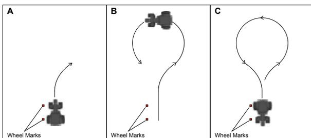
2. Stop the vehicle in the exact same location shown by the previously set marks so that the rear tires are now over the marks of the front tires or the centre of the track is at the same point but in the opposite direction.
