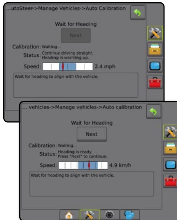
*NOTE: If the orientation has been set incorrectly, the FieldPilot Pro system or UniPilot Pro system will not be able to accurately determine a heading. Drive the vehicle forward for 150 m and then restart the calibration.*
