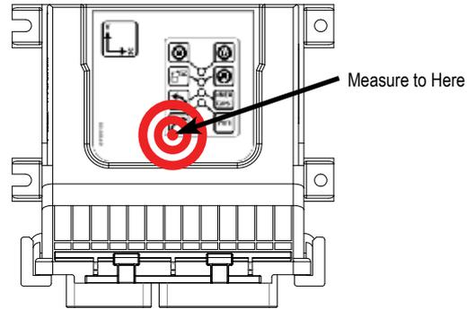
NOTE: The bull's eye is not printed on the actual SCM Pro unit. It is shown here only to indicate the location of the measurement point on the SCM Pro.
