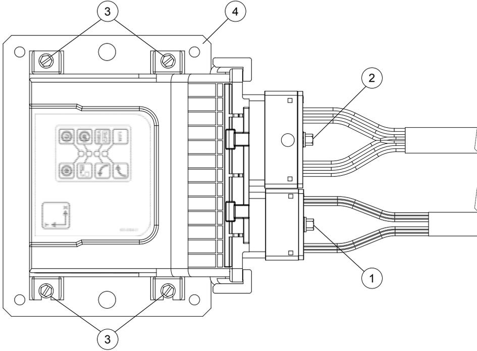
The figure above shows SCM Pro installed on the metal bracket with main and vehicle specific harnesses connected.
