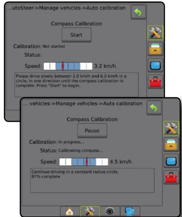
4. During the compass calibration process the system will display a progress indicator in percentage. Continue driving in a circle until the compass calibrates and the next calibration screen appears.
