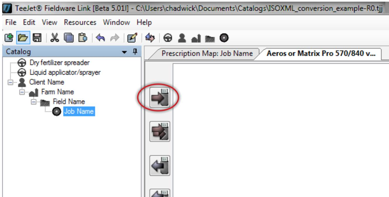
The job and appropriate Machine profile will now show in the right pane. Be very careful to click on the 'Done' button in the lower right corner of the right pane before removing the USB drive from the computer.
