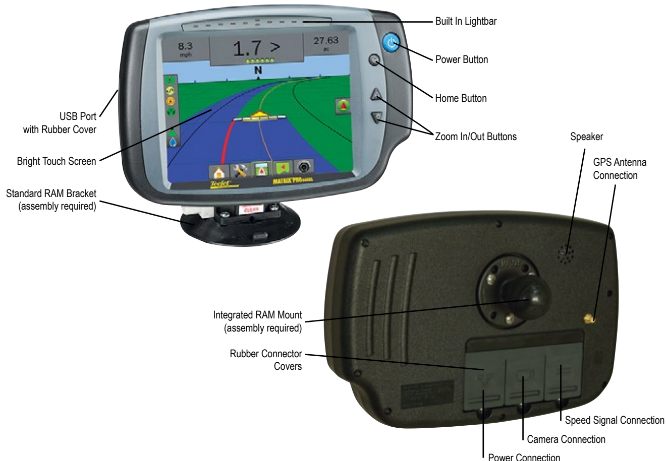
Figure 1-2: Matrix Pro 840GS Console Front and Back
