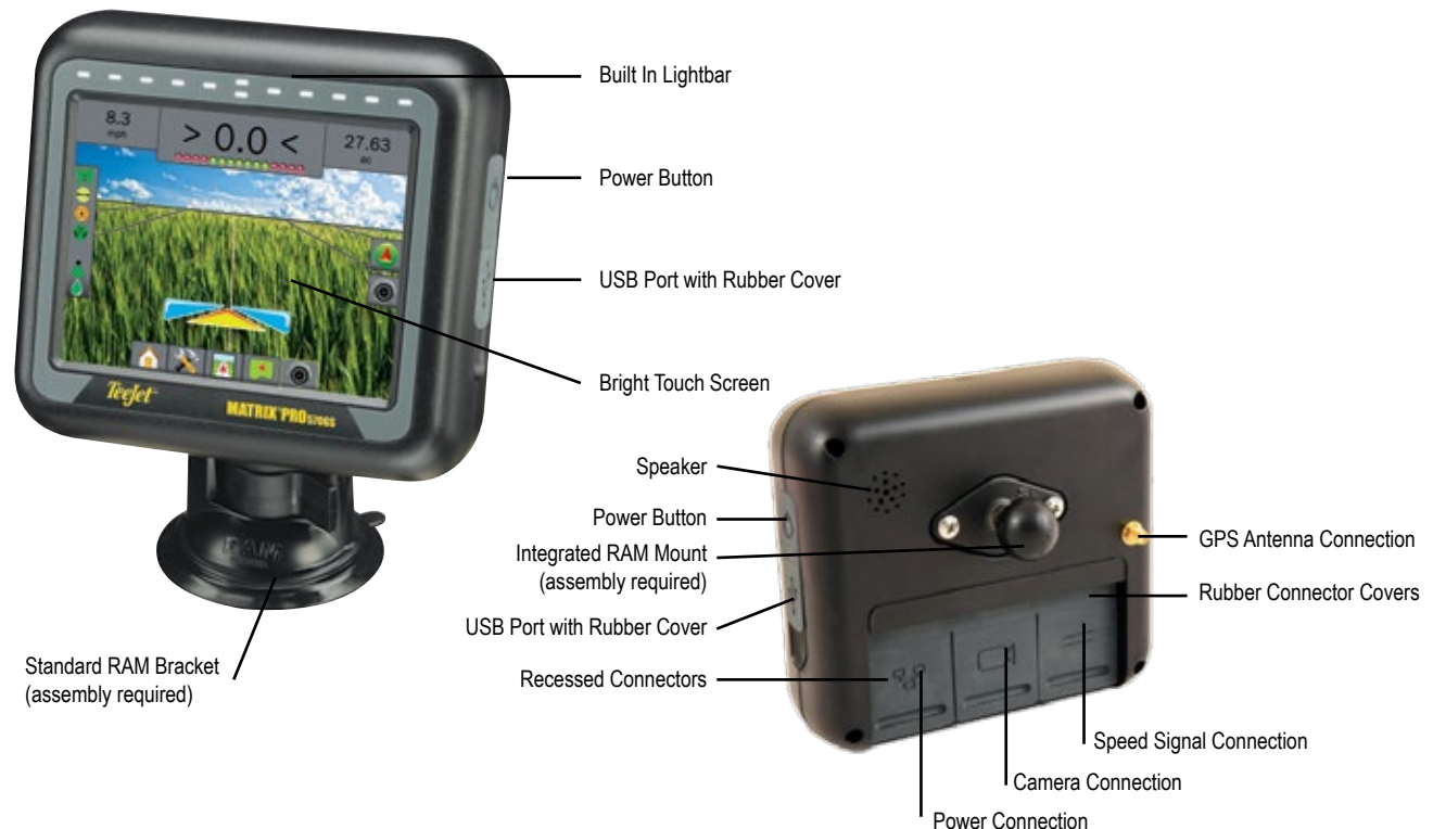
Figure 1-1: Matrix Pro 570GS Console Front and Back
