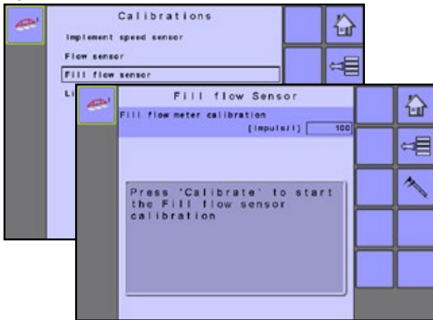
Figure 3-22: Fill flow sensor
