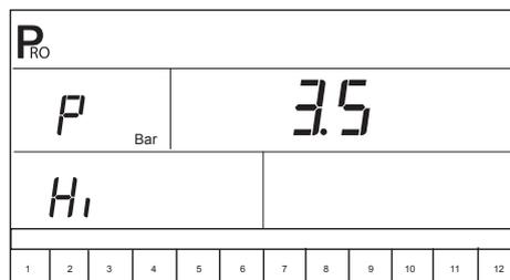
NOTE: If a pressure transducer is not installed on the system, skip this step by pressing the Programme
