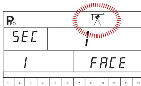
Use the Plus  $\oplus$  or Minus  $\ominus$  keys to adjust the value. This step will repeat for each section. Press the Programme  $\text{P}$  key to advance to the next section. The number of sections available is determined within the OEM setup options.
