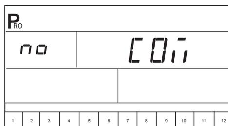
If the 844-AB has not been upgraded with the communication package, no change is required. If a change is necessary, press the Plus  $\oplus$  or Minus  $\ominus$  keys to select the type of communication used. Press the Programme  $\text{P}$  key to accept the value and advance to the beginning of System Setup mode.
