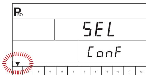
Press the Auto/man  $\leftrightarrow$  key to setup the reference pressure and reference flow of the selected preset.
