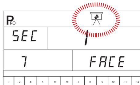
After cycling through all sections, press the Programme  $\text{P}$  key to advance and return to the first programme step.
