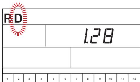
Use the Plus  $\oplus$  or Minus  $\ominus$  keys to change the value. Press the Plus  $\oplus$  and Minus  $\ominus$  keys simultaneously to clear the value to “0”. Press the Programme  $\text{P}$  key to accept the value and advance to the next step.
