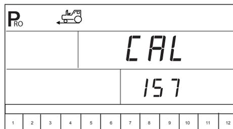
**NOTE:** Once the automatic speed calibration process has been activated, no other functions will operate until the console receives speed impulses for calibration. To deactivate automatic calibration mode, press the Plus (+) key twice.
