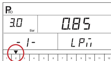
Once programming is complete for all presets, press the Programme  $\text{P}$  key to advance to the next programming step.
