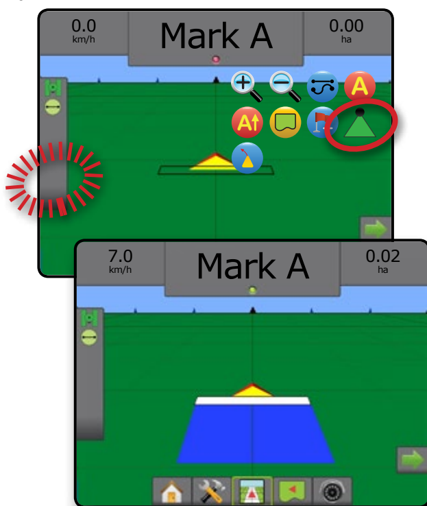
Figure 6-40: All booms off/on – No SDM
