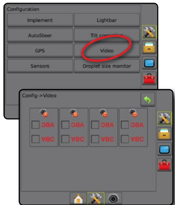
Figure 5-15: Video with 4 channel VSM
