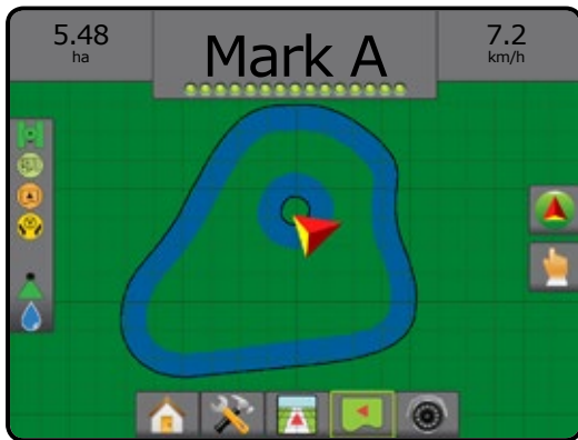
Figure 6-34: Add interior boundary
