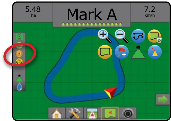
Figure 6-36: Finish boundary – Travel to starting point
