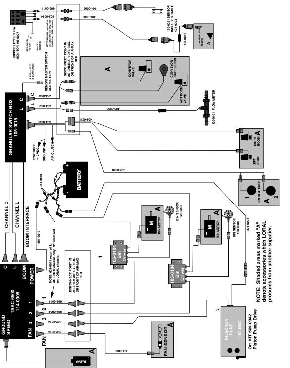
TASC 6500 ON LORAL AIR MAX WITH THE WET BOOM OPTION, ONE INJECTION PUMP AND TWO GRANULAR COAPPLICATOR BINS ON THE CONVEYOR.
