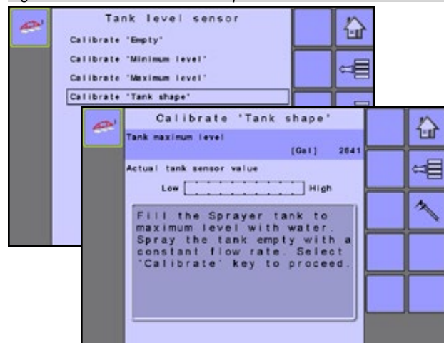
Figure 3-32: Calibrate "Tank Shape"
