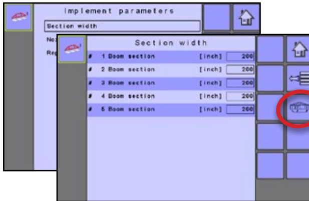
Figure 3-12: Boom Section Width
