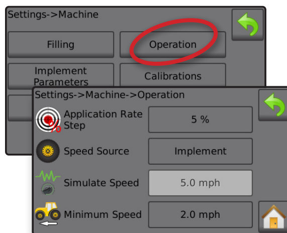
Figure 11: Application Rate Step On Operation Screen
