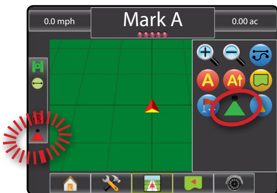
Figure 1-26: Automatic to All Sections On Mode
