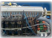
Connect loose wires to the connection bloc. Below a informative table but verify that the respective connections are giving out 12 V when section is ON.
