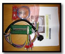
If the DP Tronic controller has no BoomPilot interface installed from the factory or the BoomPilot interface installed, is of an older type than described above, it's necessary to install Berthoud no. 292 483 or TeeJet no. 902-422, before using Teejet kit no. 990-888 or 990-889.
