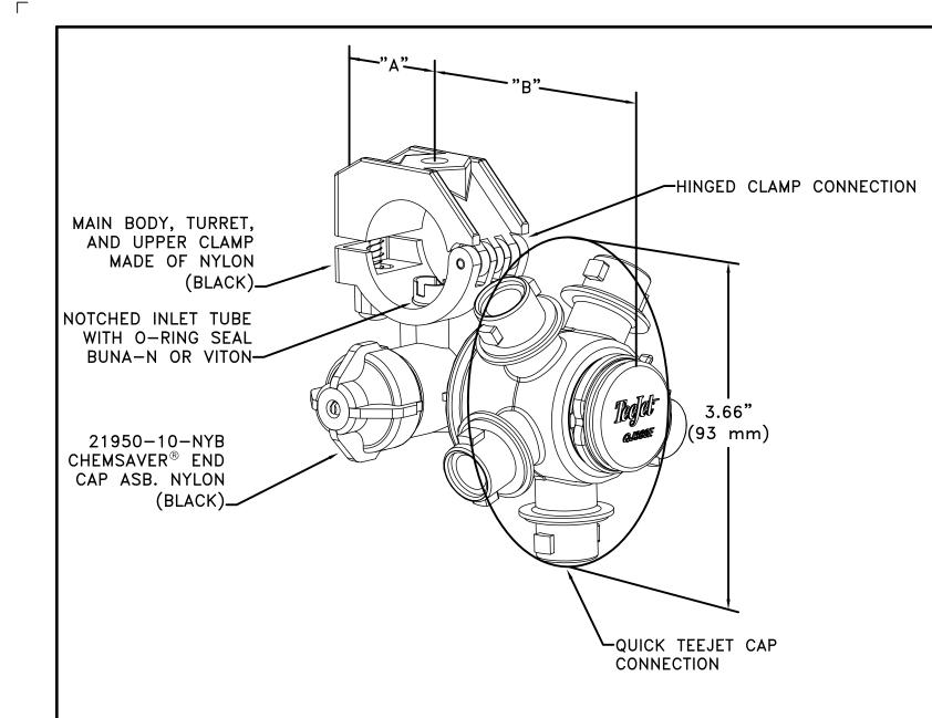
TO INSTALL ASSEMBLY DRILL 3/8" (9.5 mm) DIAMETER HOLE IN PIPE, DEBURR, THEN INSERT NOZZLE BODY INLET AND CLAMP ASSEMBLY IN PLACE.
