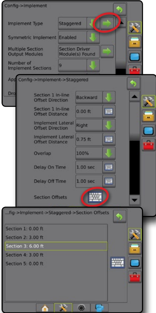
Figure 6-24: Offset Directions and Distances – Behind Section 1
