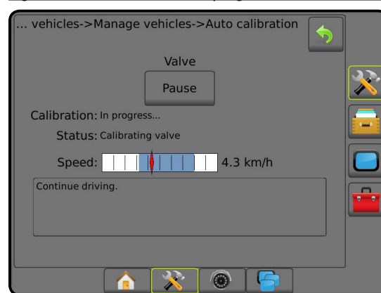
Figure 26: Valve calibration in progress
