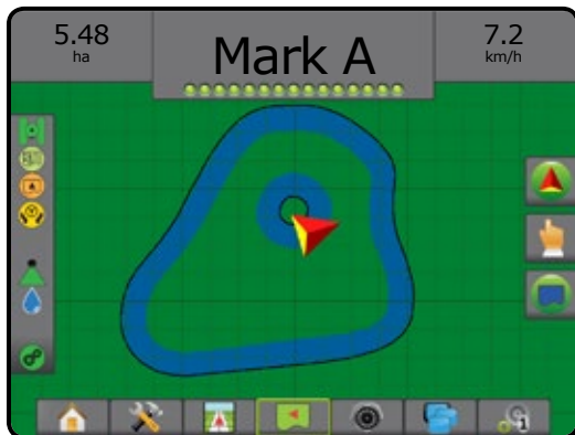
Figure 7-34: Add interior boundary
