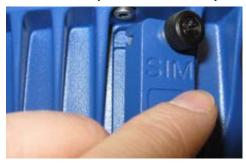
2. Install the SIM following the orientation shown on the SIM cover (notch up and in, as shown).
