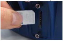
The SIM connector is a push-in/push-out type. If the SIM is correctly installed, its outside edge will be essentially flush with the surrounding enclosure metal surface.
