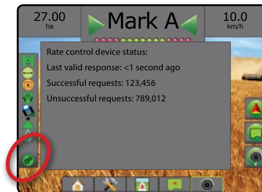
Figure 8-5: Product rate control status
