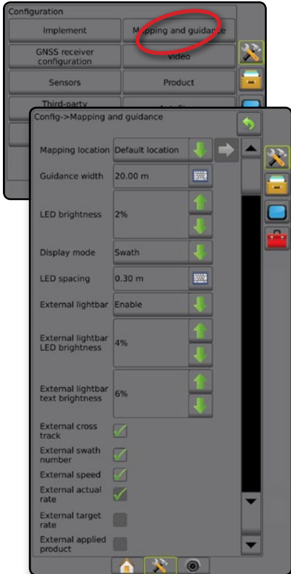
Figure 4-13: Mapping and guidance with external lightbar
