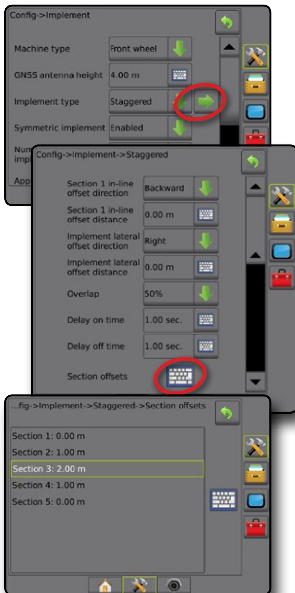
Figure 6-19: Offset directions and distances – behind section 1
