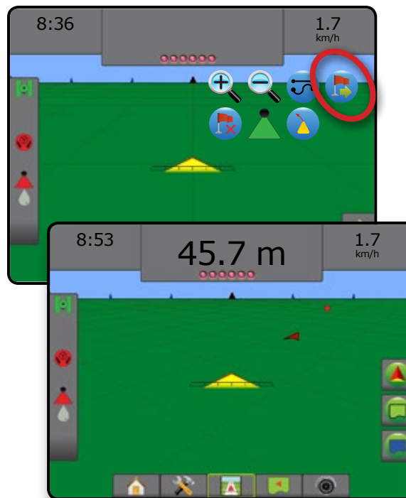
Figure 7-22: Return to point guidance – Vehicle view
