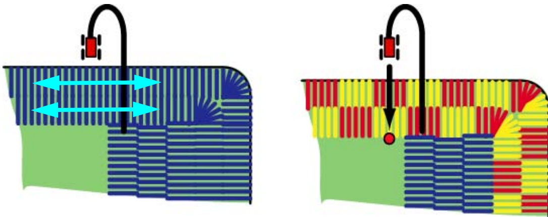
Figure 4-23: Crossing through Headlands
