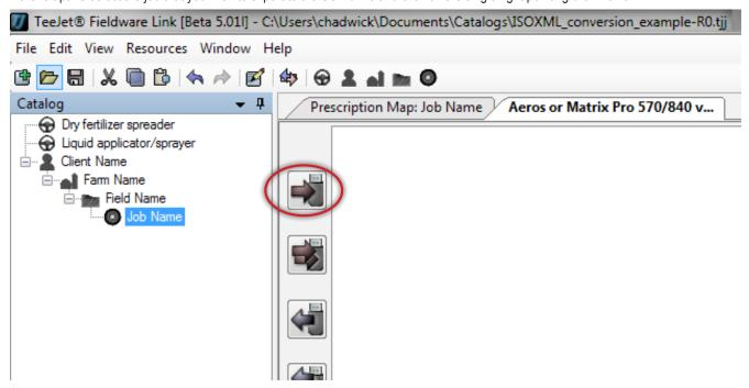
The job and appropriate Machine profile will now show in the right pane. Be very careful to click on the 'Done' button in the lower right corner of the right pane before removing the USB drive from the computer.
