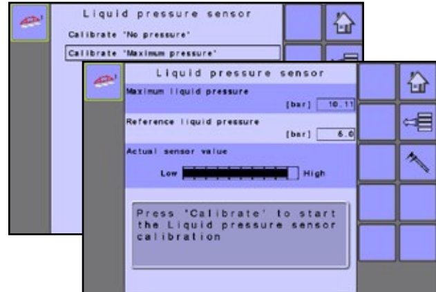
Figure 3-20: Calibrate “Maximum pressure”
