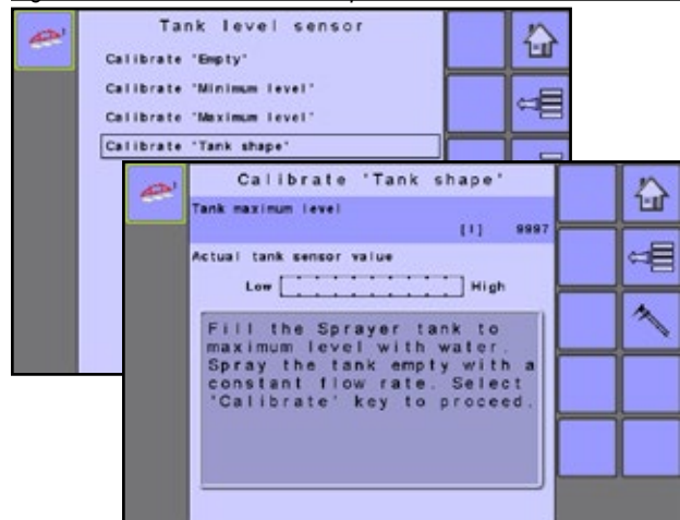
Figure 3-32: Calibrate “Tank shape”
