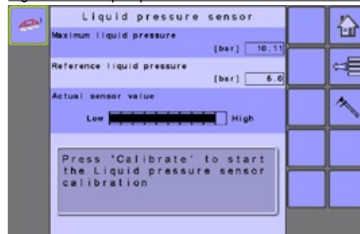
Figure 3-21: Liquid pressure sensor calibration
