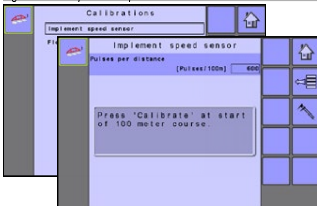
Figure 3-16: Implement Speed Sensor
