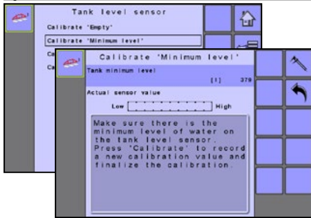
Figure 3-28: Calibrate “Minimum level”
