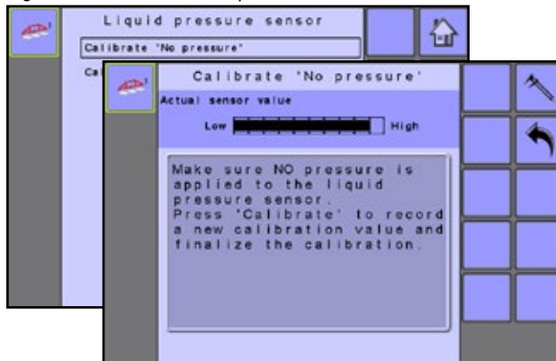
Figure 3-19: Calibrate “No pressure”
