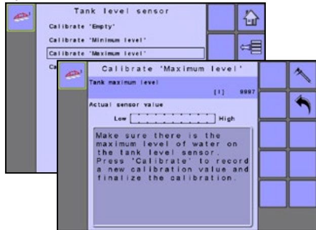
Figure 3-30: Calibrate “Maximum level”
