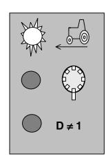
The Press alarm LED flashes when the signal from the pressure sensor drops below 4mA while spraying (Master in the ON position). This indicates that the pressure sensor is not working properly.
