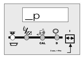
The display will then display a flashing flow rate represented in I/min at 2 bar. The Tip Select LED will also be flashing. Use the + and keys to adjust this value so that it matches the flow rate of one of your tips in I/min at 2 bar.
