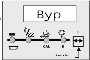
Note: This setting must match the actual plumbed mode of the regulating valve. Changing this setting will only reverse the polarity to the valve, it will not effect the physical operation of the valve.
