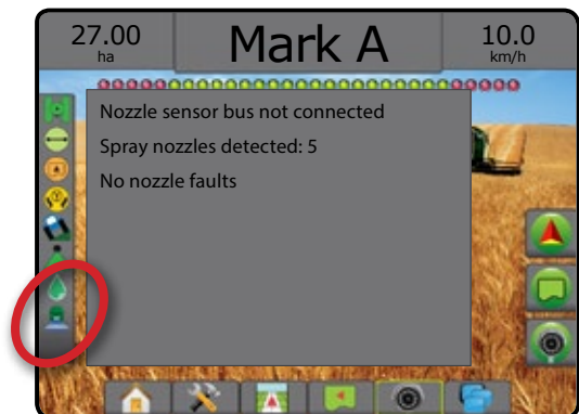
Figure 7-13: Nozzle flow status
