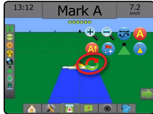
Figure 7-33: Nozzle Flow Monitor
