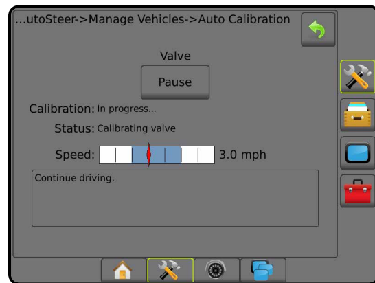
Figure 26: Valve Calibration in Progress
