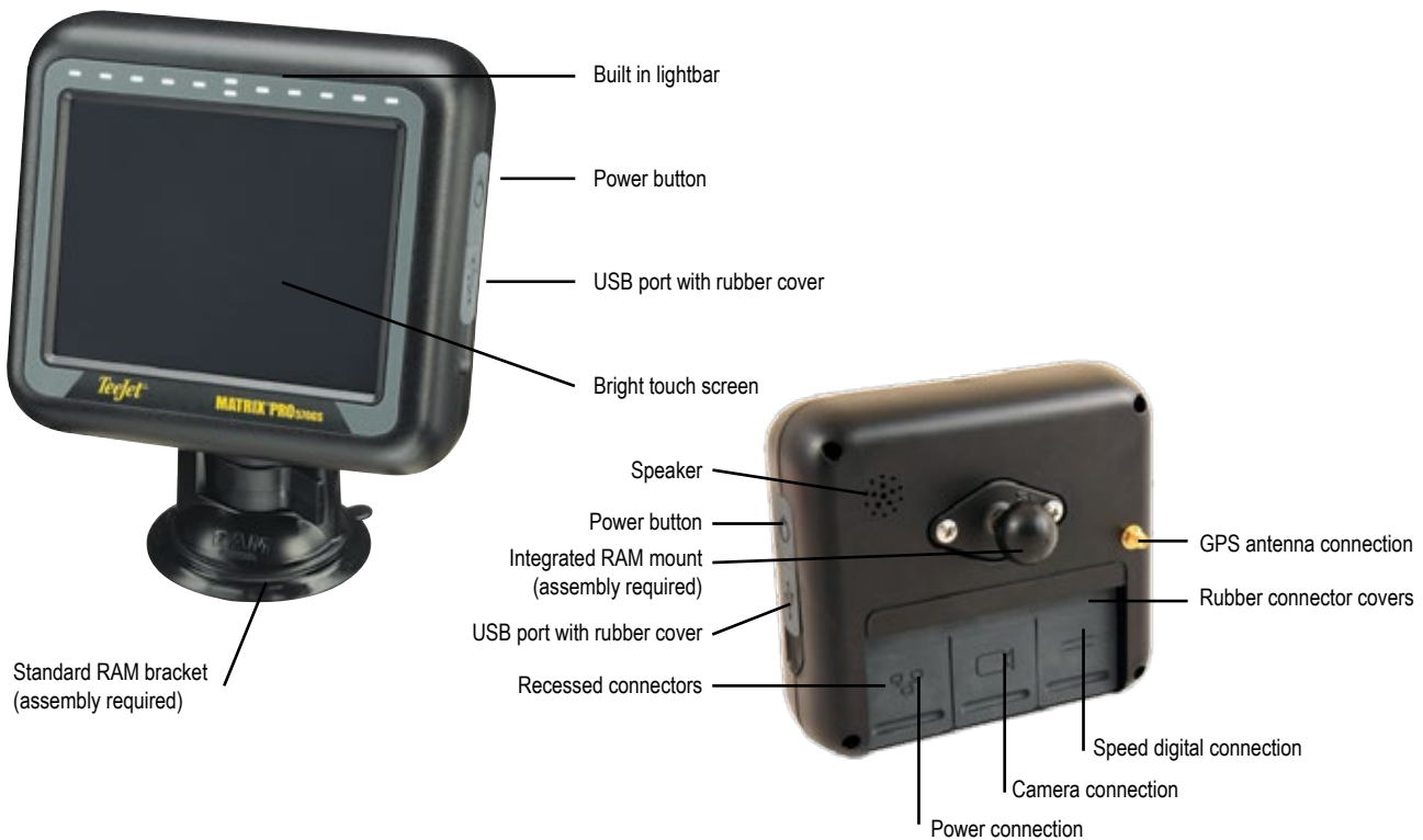
Figure 1-1: Matrix Pro 570GS Console Front and Back
