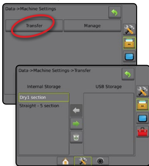
Figure 4-35: Machine Settings – Transfer
