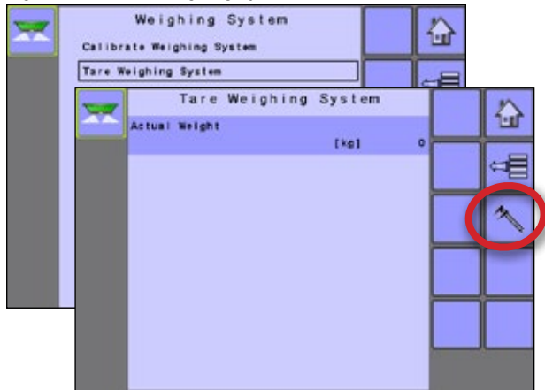
Figure 3-25: Tare weighing system
