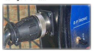
Make a hole in the left part of the plastic housing and install the round connector. The Hole should be Ø25 mm and fixing holes Ø3.2 mm.
