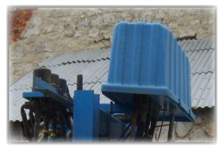
Fix the relay box to the frame
