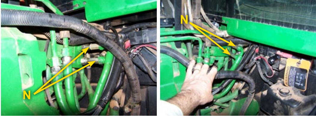
Figure 1-12: Install the Left and Right Steer Hoses
