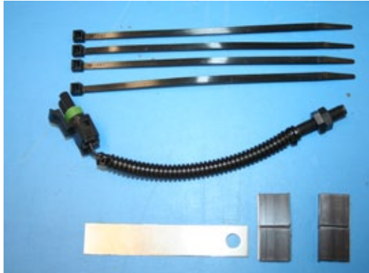
Figure 1-15: Install Steering Disengage Switch (Kit 91-07011)
