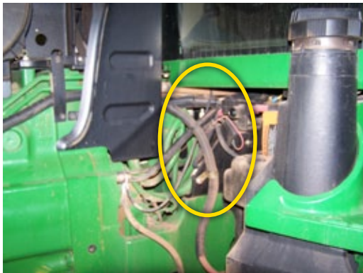
Figure 1-11: Install the Left and Right Steer Hoses
