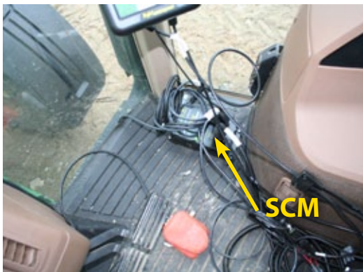
Figure 1-17: Recommended Electronics Installation
