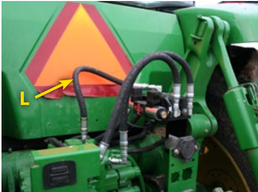
Figure 1-8: Install The LS Hose and Adapter
