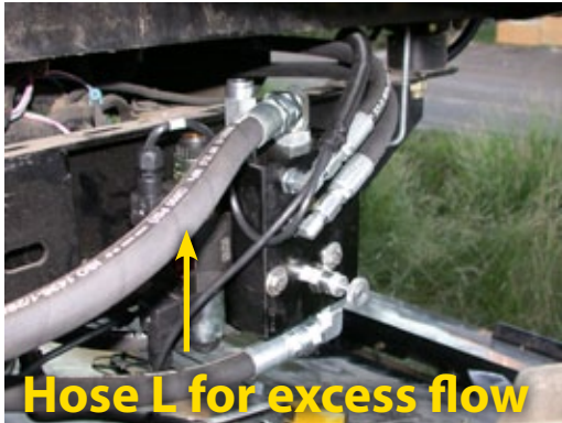
Figure 1-7: Install Excess Flow Hose
