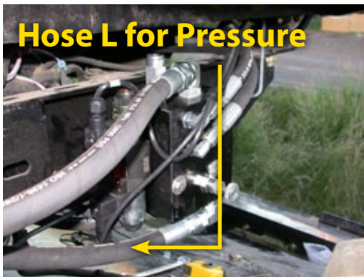
Figure 1-8: Install Pressure Hose
