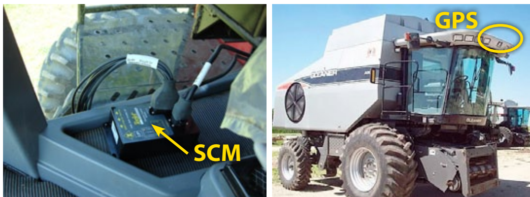
Figure 1-14: Recommended Electronics Installation
