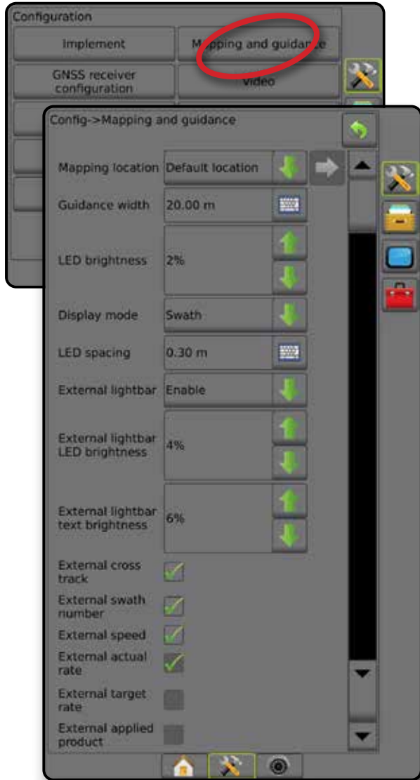
Figure 4-13: Mapping and guidance with external lightbar
