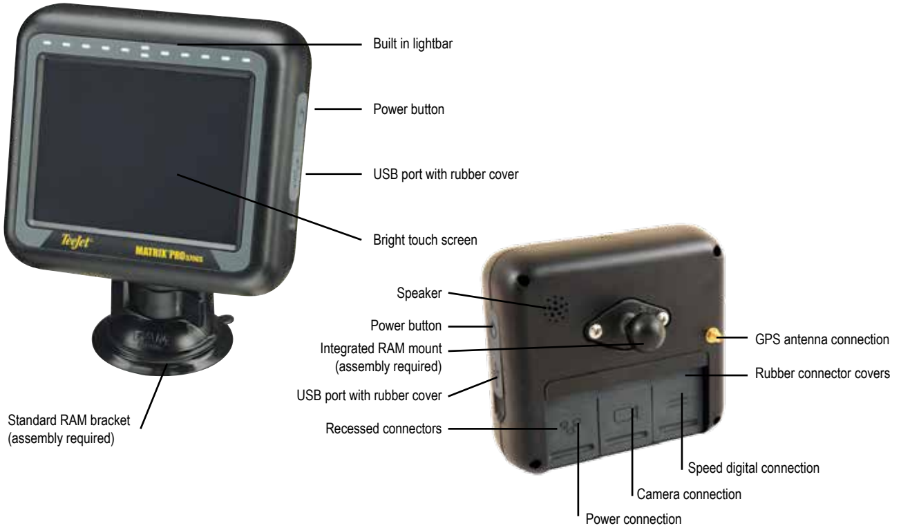
Figure 1-1: Matrix Pro 570GS console front and back
