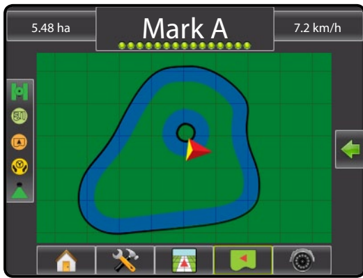
Figure 7-56: Add Interior Boundary
