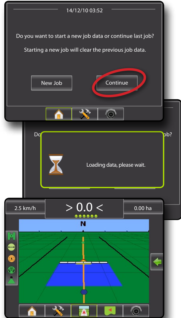
Figure 4-8: Continue the Existing Job
