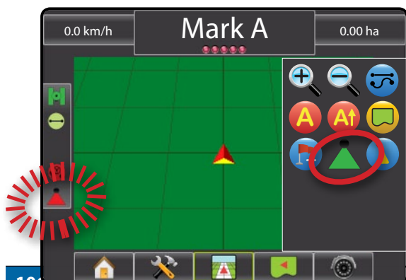
Figure 7-62: Automatic to All Sections On Mode
