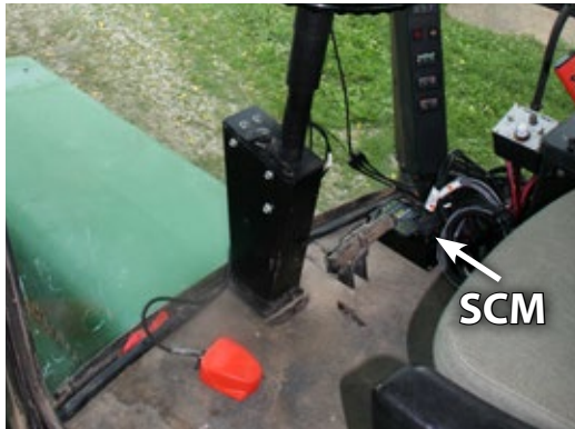
Figure 1-14: Recommended Electronics Installation
