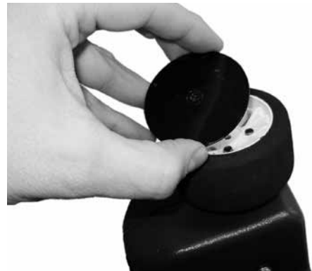
Figure 1-22: Contact Wheel With Holding Pins
