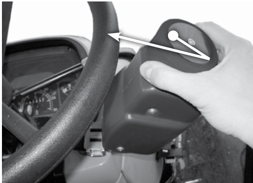
Figure 1-16: Pull UniPilot ESM to Operation Position
