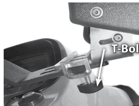
Figure 1-7: Secure the Mounting Bracket
