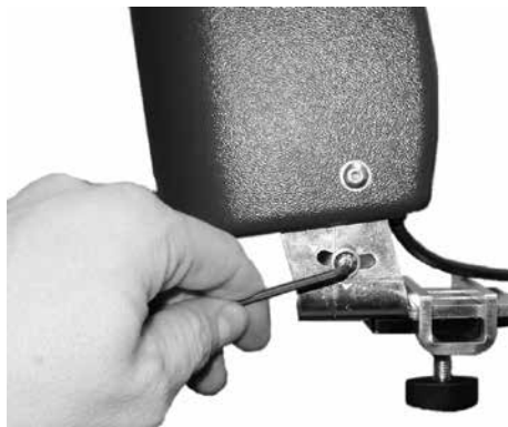
Figure 1-18: Loosen Mounting Bracket Screws
