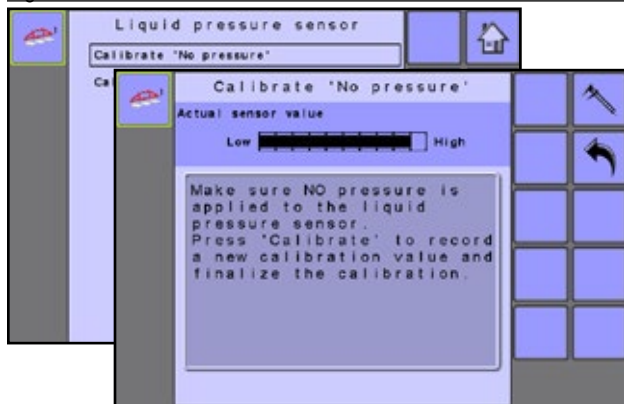
Figure 3-19: Calibrate “No Pressure”
