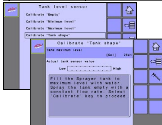
Figure 3-32: Calibrate "Tank Shape"
