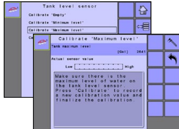
Figure 3-30: Calibrate "Maximum Level"
