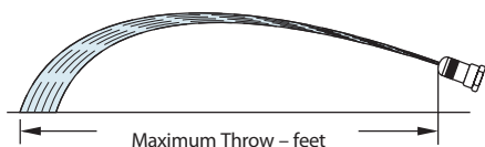
TIP SETTING "B" STRAIGHT STREAM SPRAY PATTERN
