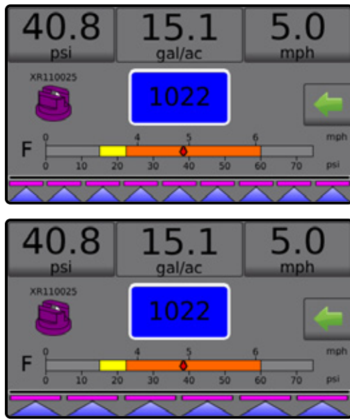
Figure 3-41: Operation Screen with 9 or 6 Sections
