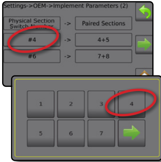
Figure 3-43: Physical Section Switch Number
