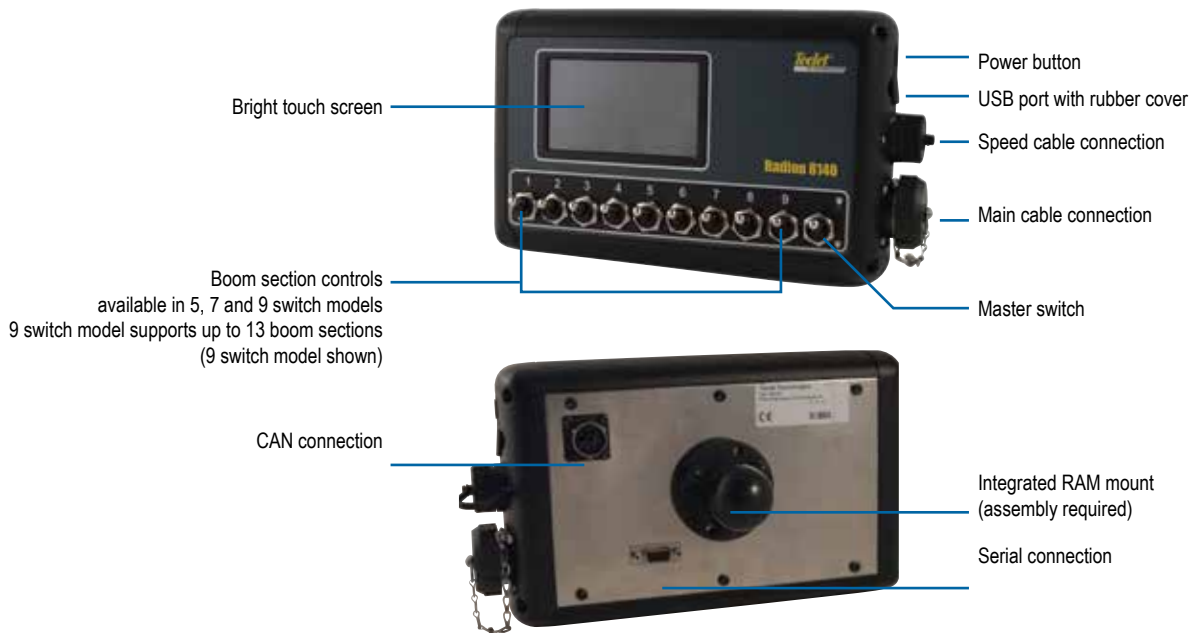
Figure 1-1: Radion 8140 console front and back
