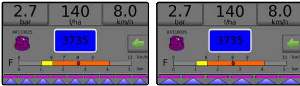
Figure 3-41: Operation screen with 9 or 6 sections
