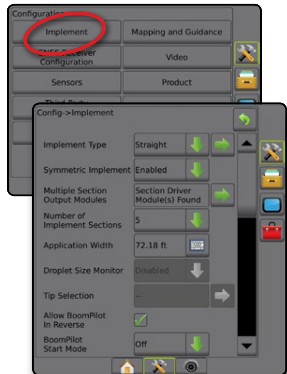
Figure 4-7: Implement – Multiple Sections with SDM or SFM Setup
