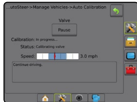
Figure 26: Valve Calibration in Progress
