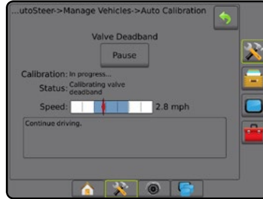
Figure 24: Valve Deadband Calibration in Progress
