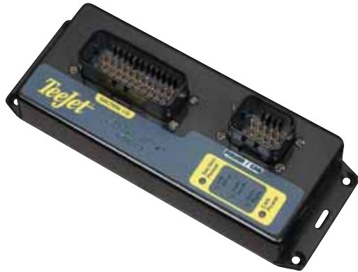
Figure 1-10: Sections Driver Module
