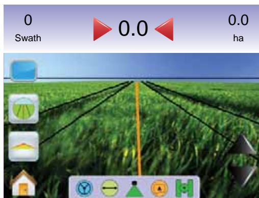
Figure 3-59: VSM Not Installed
